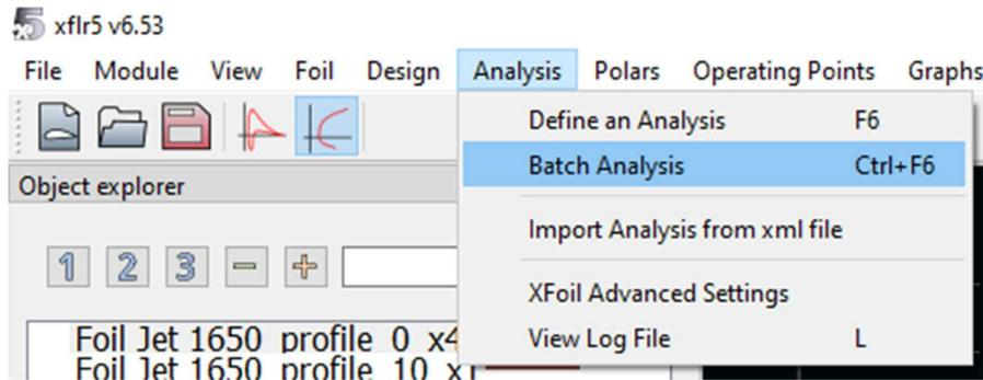
Then select all the profiles, and launch the Type 1 analyzes between  $-5^\circ$  and  $20^\circ$ :
