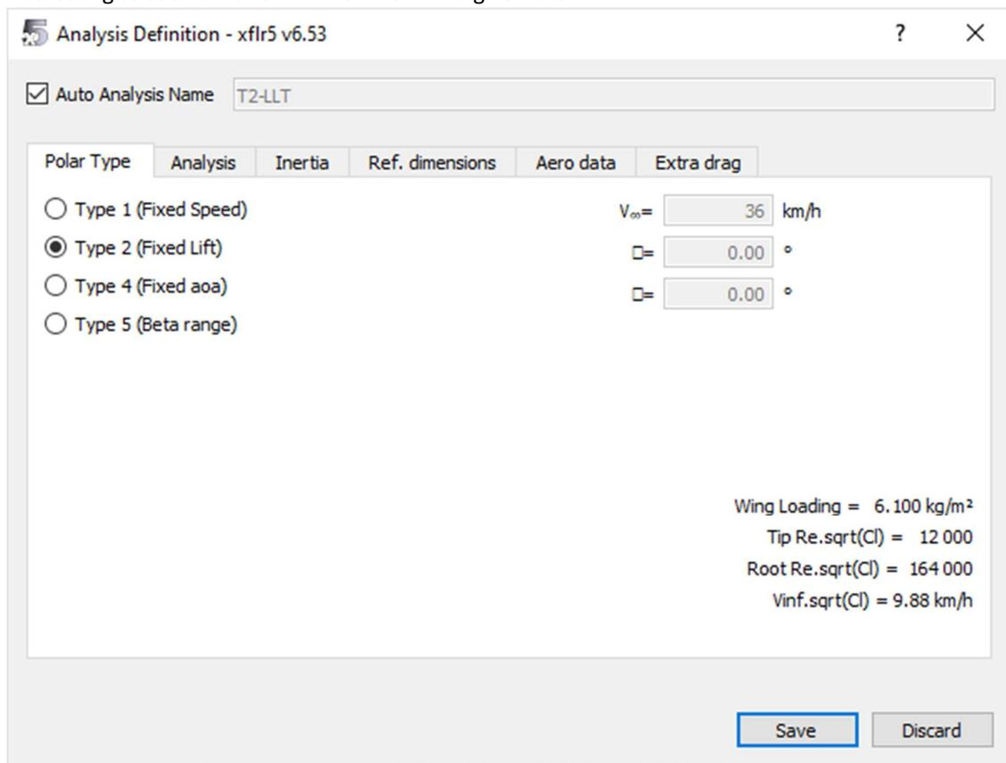
You must then choose the method in the Analysis tab. Ring vortex works well. We're not going to check Viscous just yet, which will allow us to get lift faster.
