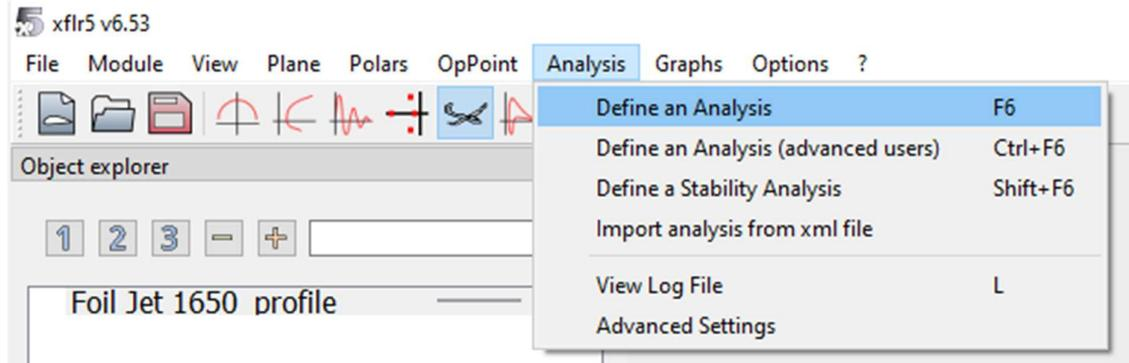
You can do an analysis at a given speed (Type 1), or at a given lift (Type 2). The Type 2 analysis is very interesting to see how a foil will behave with a given user:
