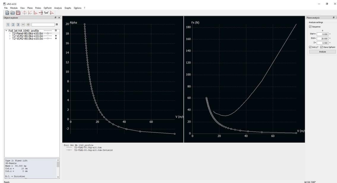
We can see here that the bank at 10 kt is not 2 ° but 4 °. We descend to 2 ° around 12 kt. The minimum drag is around 14 kt, and the optimum range between 12 kt and 16 kt.
