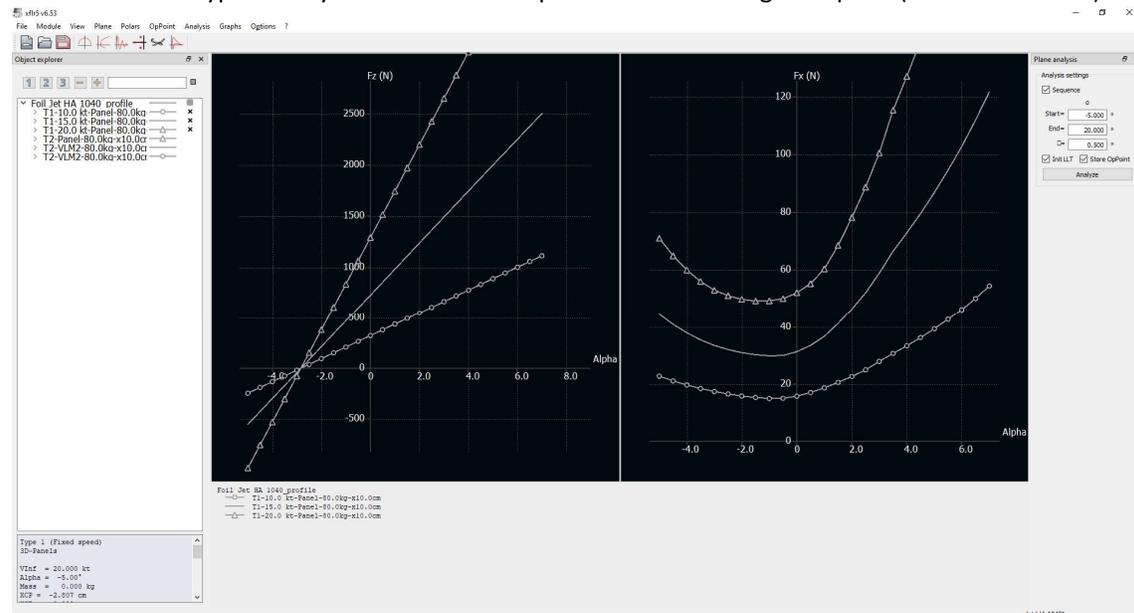
It is also possible to load the stab to have lift and overall drag.
