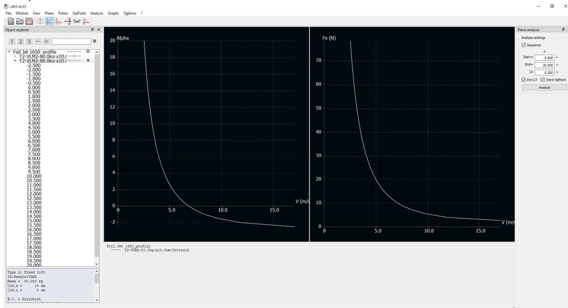
This analysis calculates for each inclination of the foil (here between  $-5^\circ$  and  $20^\circ$ ) the speed it takes for the foil to carry  $80\text{ kg}$  (a lift of  $784\text{ N}$  therefore). You can also display the drag  $F_x$  for each speed (with the inclination that corresponds to it).
