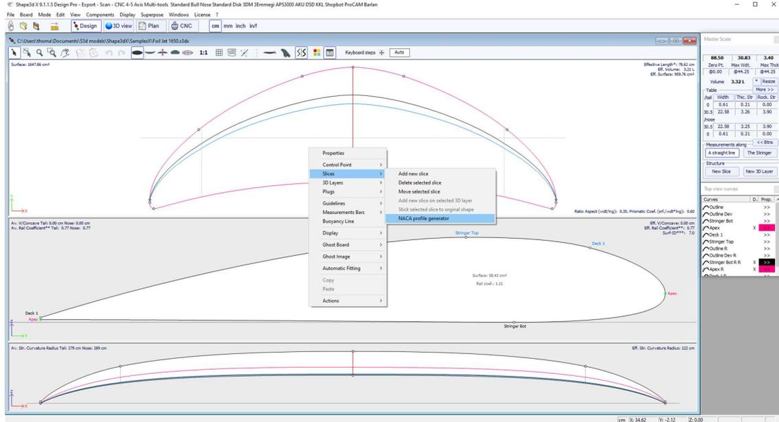
This function allows you to adjust a slice on a NACA profile (or another profile imported from a .dat file), but also to export the foil so that it is easy to analyze in Xflr5.
